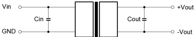
Figure 1. Typical external circuit
